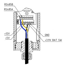
Connect the black wire to the correct supply voltage according to the specification of the KELLER sensor, in this example "+3.9 V" (Pin 11) and the white wire to GND (Pin 12).
